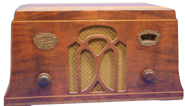
Zenith Model 705 Radio – This is a 6 tube radio manufactured in 1933. Cabinet made of wood. Covers the AM frequency band. Daniel Schoo, De Kalb, IL
