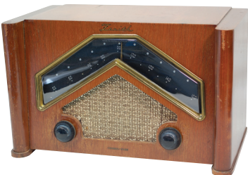
Zenith Model 705 Radio – This is a 6 tube radio manufactured in 1933. Cabinet made of wood. Covers the AM frequency band. Daniel Schoo, De Kalb, IL
