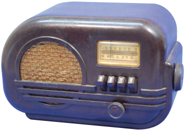
Emerson Model FG-330 Radio – This Bakelite radio was made in 1941 and extremely popular. The chassis contains 5 tubes. Daniel Schoo, De Kalb, IL
