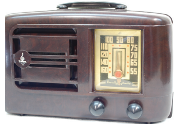
Zenith Model 6D029 Radio – Made by Zenith in 1946. Had the famous V-shaped black dial. Could be powered by both AC and DC. Daniel Schoo, De Kalb, IL
